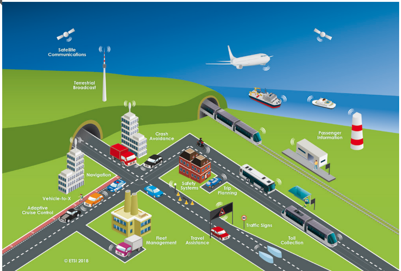
Fig. 4 Complete Concept of an Intelligent Transport System (ITS) according to ETSI
